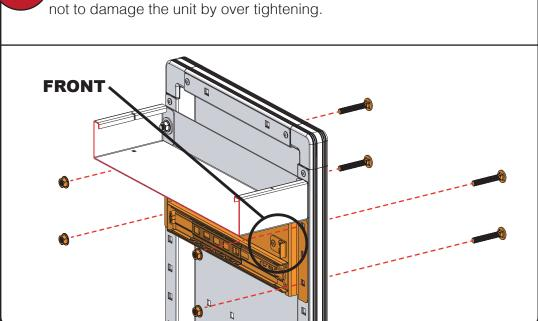
Secure the right fixing panel (AS3506) to the side panel using M8x50
