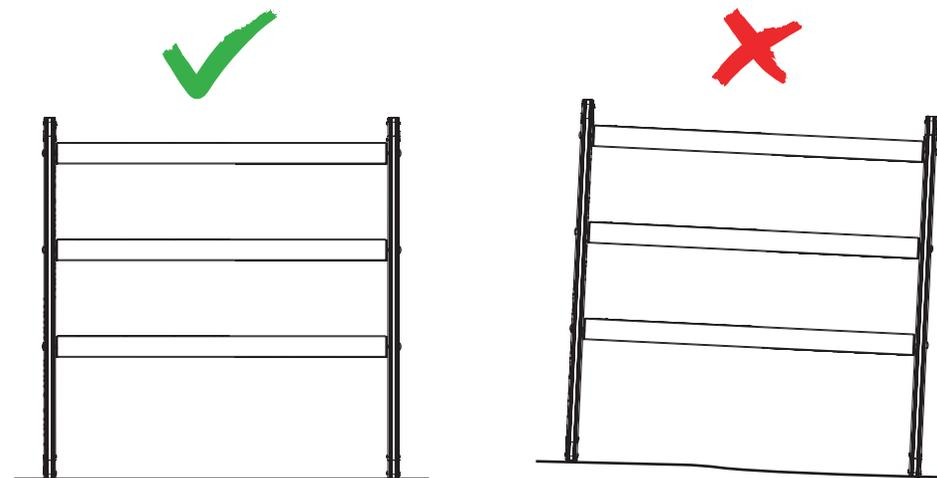
**03** Assemble the racking unit, leaving space for the drawer(s) following instruction manual IN8377.
