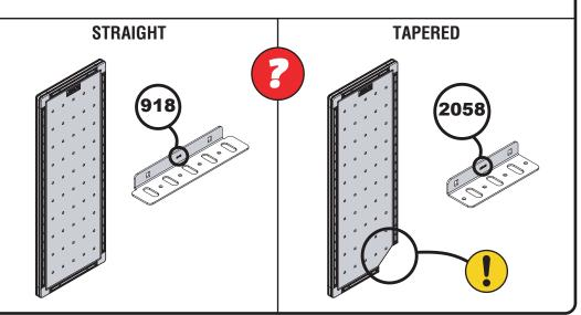
Secure the floor brackets to the side panels using M8x50 coach bolts, M8 washers and M8 flange nuts. Tighten all fixings to 5Nm. Take care not to damage the unit by over tightening.
