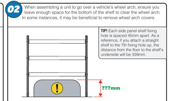
If you are also installing a drop-down door, do not position a shelf below the 7th fixing hole. You can install the drop-down door once the shelves are fully assembled.
