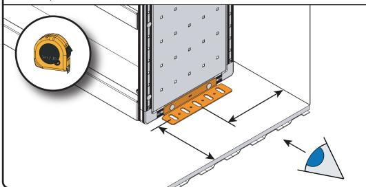
After ensuring the area under the floor bracket / vehicle floor is free from obstruction, mark the hole centres of the fixing slots you have chosen to use. Move the unit to one side and drill Ø8.5mm through the floor of the vehicle (three positions for each bracket).
