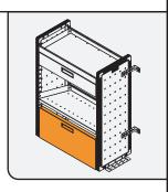
If you are also installing a drawer, ensure that you plan to leave enough space. Drawers can be positioned anywhere on the unit and one drawer requires the space of three side fixing holes as illustrated. You can install the drawer once the shelves are fully assembled.
