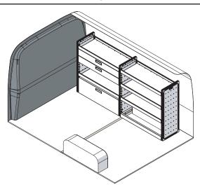
If you are fixing a straight side panel, use floor bracket ME0918. If you are fixing a tapered side panel, use floor bracket ME2058.
