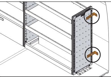
Secure the fixing brackets (ME0919) to the unit in the required positions using M8x50 coach bolts, M8 washers and M8 flange nuts. If required, an extension bracket can be used as shown in step four.
