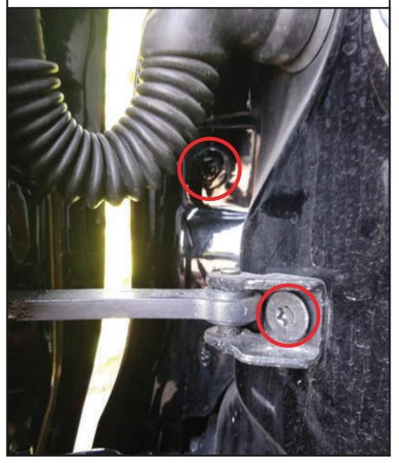
Hold the loom guard in place lining up the holes with the removed bolt and torx screw and re-attach.
