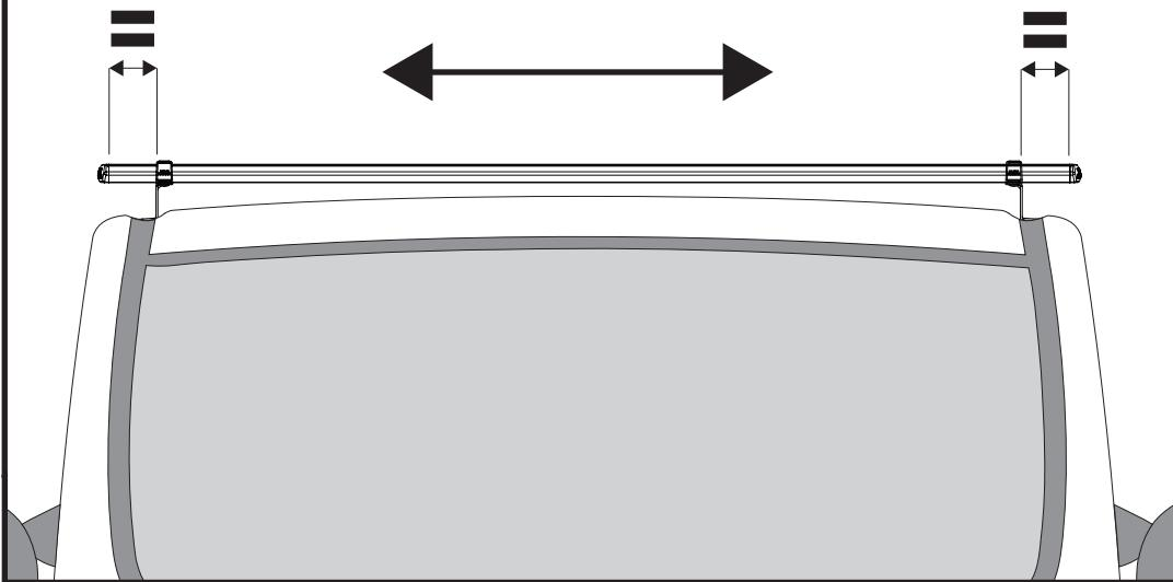
**7** Tighten the roof bar fixings to 11Nm.
