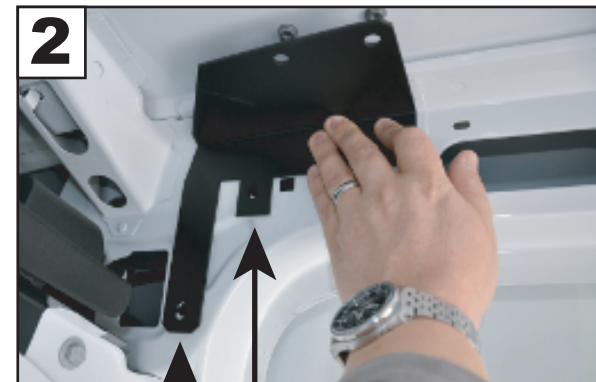
M6 1/4 TURN NUT INSERT LOCATIONS
