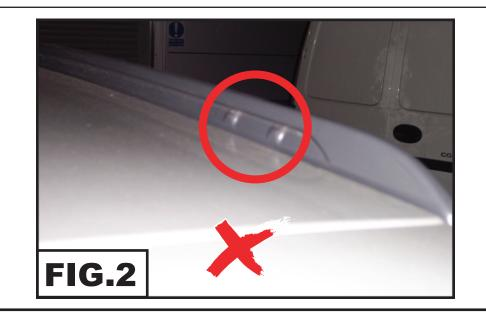
**3** Position the side rails on the **inside** of the vehicle rail and measure 225mm from closed tailgate door to the centre of the rear fixing hole. Once the side rail is in position carefully push it down into the gap between the factory fitted side rail and the roof to allow correct fitting of the clamps in step 4.
