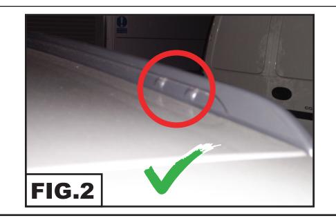
**3** Position the side rails on the **outside** of the vehicle rail and measure 210mm from closed tailgate door to the centre of the rear fixing hole Once the side rail is in position carefully push it down into the gap between the factory fitted side rail and the roof to allow correct fitting of the clamps in step 4.
