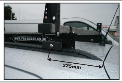
4 Insert fixing brackets into the roof rail channel and loosely secure the side rails onto the **inside** of the vehicle rail as shown below using M6x40 coach bolts, M6 washers & M6 serrated nuts. Ensure that the top hat flange is facing inwards.
