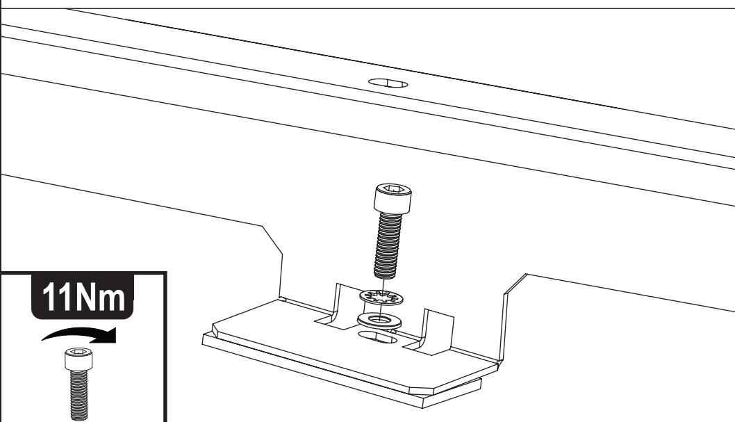
**5** Place roof bars onto the side rails with the t-track facing upwards and loosely secure using top hat brackets, M6x16 coach bolts & M6 serrated nuts.
