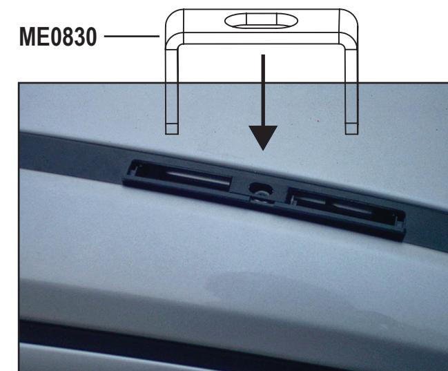
**4** Secure the side rails to the fixing points using M6x20 allen bolts, M6 shakeproofs & M6 washers. Ensure that the top hat flange is facing inwards.
