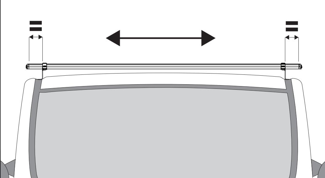
**7** Tighten the roof bar fixings to 11Nm.
