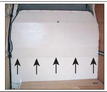
Once happy with the position of the bulkhead carefully drill 4.5mm through the bottom sections fixing holes in the positions shown below and secure using No14x1/2" self tap screws (FX4087). (5 positions along the bottom and 4 each side).
