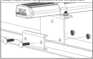
Flex the top hat covers over the top hat brackets into position as shown below. Ensure that the covers click into the front and rear of the top hat brackets.
