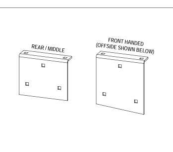
Loosely secure the roof bars onto the roof brackets using top hat brackets, M6x16 coach bolts & M6 serrated nuts. Ensure that the roof bar inserts are facing upwards.
