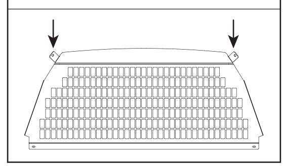
Insert M6x45 coach bolts (FX4046) through the slots into the cab area (bottom of the bulkhead) and secure M6 washers (FX4109) and M6 flange nuts (FX4016). Once in position tighten all fixings.
