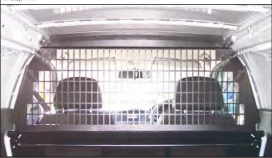
Loosely secure the bulkheads side tabs to the vehicles fixing points using M8x20 hex bolts (FX4018) and M8 shakeproof washers (FX4019).
