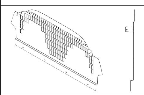
Position the bulkhead into the vehicle with the folded returns facing into the cab area and rest on the vehicles existing bottom bulkhead.
