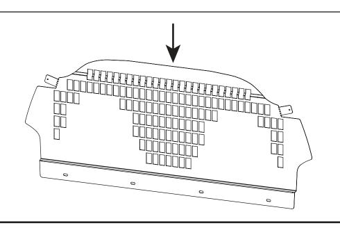
Bend the two perforated side tabs up 90 degrees (the same way as the bend in the bulkhead). Take care not to weaken the tabs by bending them the wrong way.
