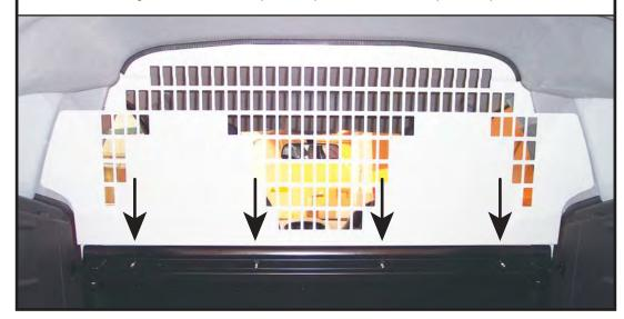
Pull the bulkhead forward towards the cab area. Once happy with the position of the bulkhead carefully drill 3.2mm through the tabs and trim and secure in place using No8x3/4" self-tap screws (FX4091).
