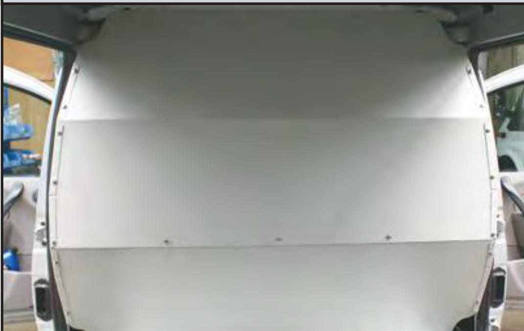
**6** Bend the side tabs inwards to suit the profile of the door pillar. When happy with the position of the tab carefully drill 4.5mm through the hole on the side tab (one per side) into the door pillar and secure using No14x1/2" self-tap screws (FX4087).
