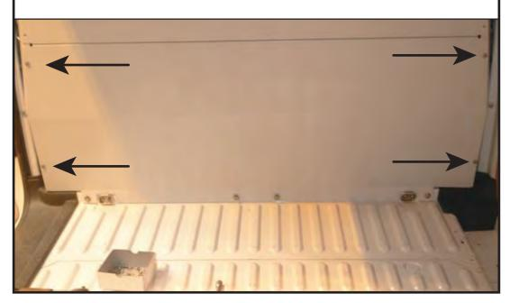
Place the top bulkhead onto the flange of the bottom bulkhead and loosely secure to the sides using M6x12 hex bolts (FX4060), M6 shakeproof washers (FX4010) and M6 washers (FX4013).
