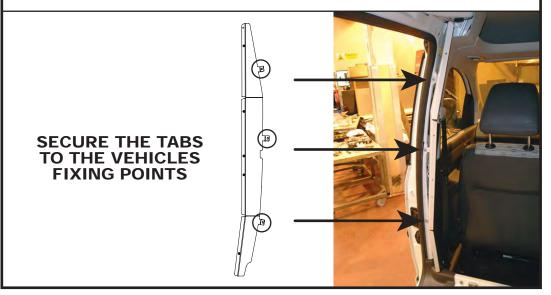
Loosely bolt the four fixing plates to the vehicles top fixing positions using M6x12 hex bolts (FX4060), M6 shakeproof washers (FX4010) and M6 washers (FX4013). Ensure that the longest face of the fixing plate is facing downwards.
