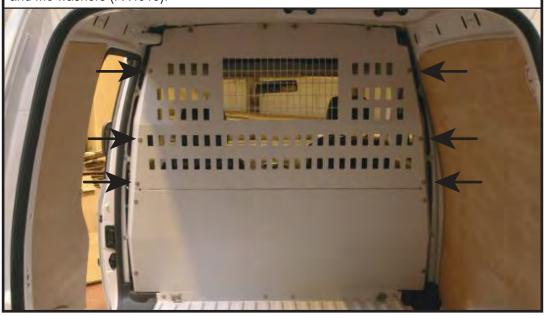
Loosely secure the top bulkhead to the four fixings plates fitted in step 3 using M6x12 hex bolts (FX4060), M6 washers (FX4013) and M6 flange nuts (FX4016). The photo below is taken from inside the cab area.
