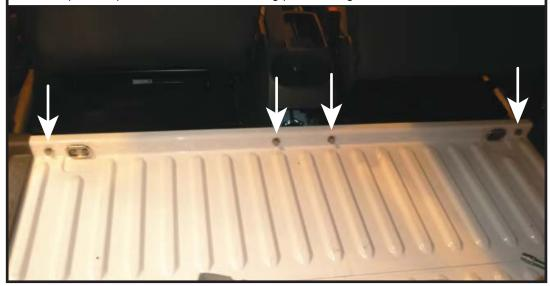
Secure both sides to the vehicles fixing points as shown below using M6x12 hex bolts (FX4060), M6 shakeproof washers (FX4010) and small M6 washers (FX4017). The sides are handed to suit both sides of the vehicle and each side has three fixing points, the photo below shows the left side.
