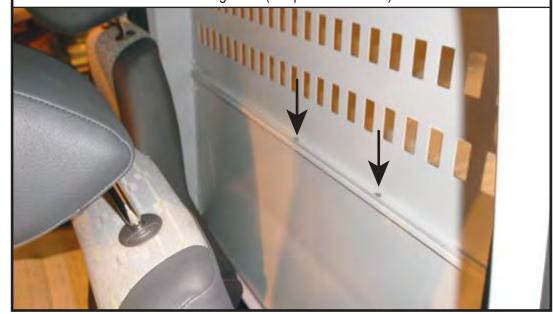
Once in position tighten all of the bulkhead fixings followed by the side fixings.
