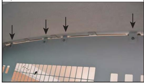
Secure the top and bottom bulkhead together using M6x16 coach bolts (FX4042), M8 washers (FX4020) and M6 flange nuts (FX4016). It may be necessary to move the seats forward to reach the fixing holes (five positions in total).
