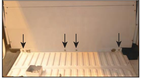
Loosely bolt the bottom bulkhead to the threaded inserts on the sides using M6x12 hex bolts (FX4060), M6 shakeproof washers (FX4010) and M6 washers (FX4013).
