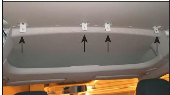
Lower the bottom bulkhead onto the four M6x16 hex bolts fitted in step 1. The bottom bulkhead has slots which fit over the bolts. Ensure that the flange on the top is facing towards the cab area.
