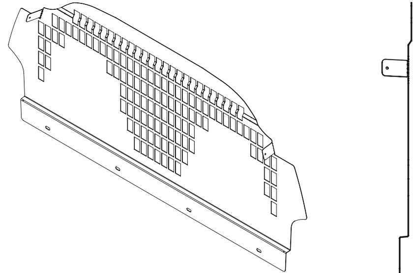
**3** Position the bulkhead into the vehicle with the folded returns facing into the cab area and rest on the vehicles existing bottom bulkhead.
