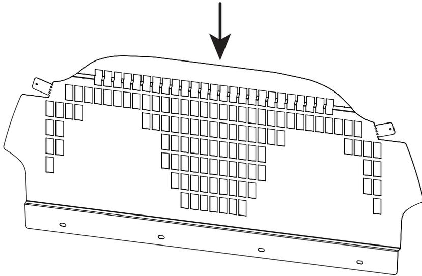
**2** Bend the two perforated side tabs up 90 degrees (the same way as the bend in the bulkhead). Take care not to weaken the tabs by bending them the wrong way.
