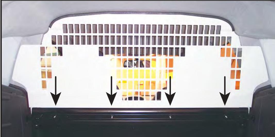
**4** Pull the bulkhead forward towards the cab area. Once happy with the position of the bulkhead carefully drill 3.2mm through the tabs and trim and secure in place using No8x3/4" self-tap screws (FX4091).
