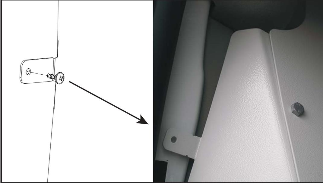
**6** Carefully drill 3.2mm through the 5 positions along the bottom flange of the bottom bulkhead and secure to the vehicle using No8x1/2" self tap screws (FX4090).
