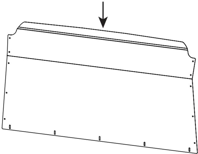
**2** Lift the bottom bulkhead into the vehicle with the bottom return facing into the load area. Place into position with the bulkhead against the passenger's seat.
