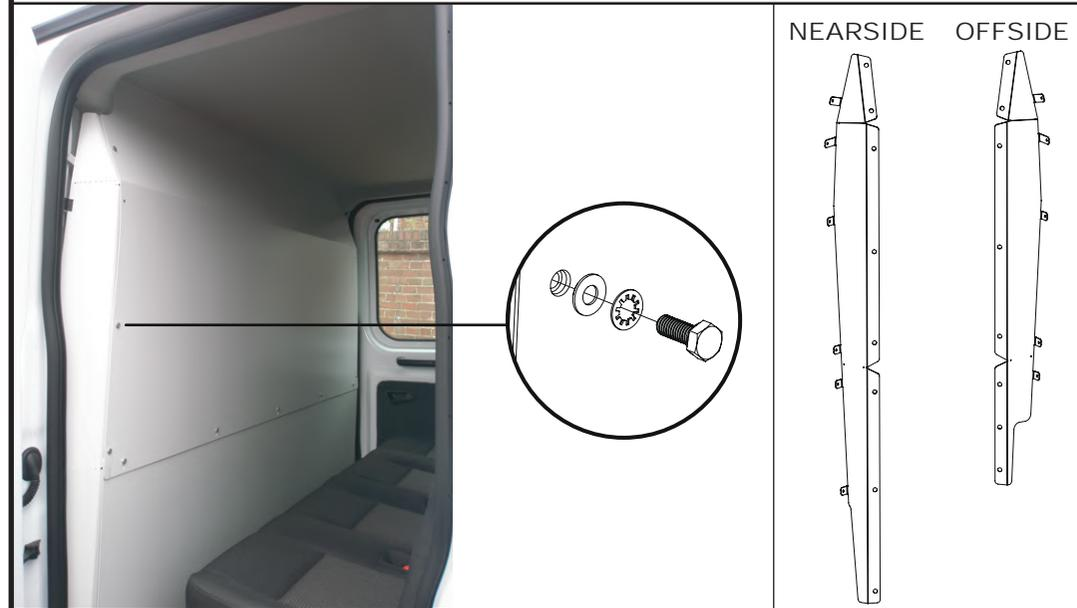
**5** Once happy with the position of the bulkhead carefully drill 3.2mm through the fixing tabs and into the vehicles 'B' pillar. Secure to the pillar using No8x1/2" self-tap screws (FX4090) (11 positions).
