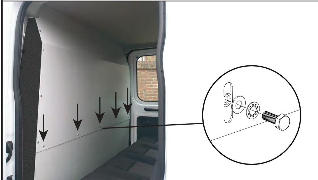
**4** Secure the sides to the bulkhead using M6x16 hex bolts (FX4012), M6 shakeproof washers (FX4010) and M6 washers (FX4017) (8 position each side). Once the sides are in position lift the top bulkhead upwards to the top of the roof and tighten all fixings.
