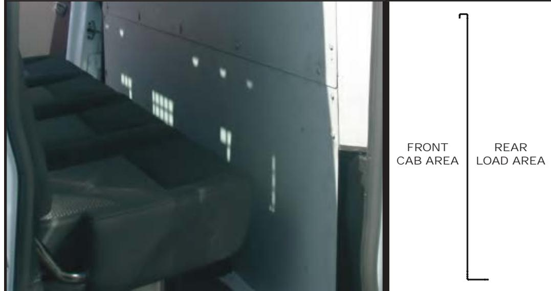
**3** Lift the top bulkhead into the vehicle and **loosely** secure to the bottom bulkhead in 5 positions using M6x16 hex bolts (FX4012), M6 shakeproof washers (FX4010) and M6 washers (FX4017).
