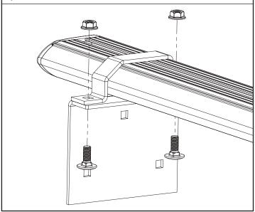
3 Slide the plastic covers on the van roof open to expose the roof fixing rail. If the van roof doesn't have plastic covers use the existing roof rail to clamp the roof brackets to.
