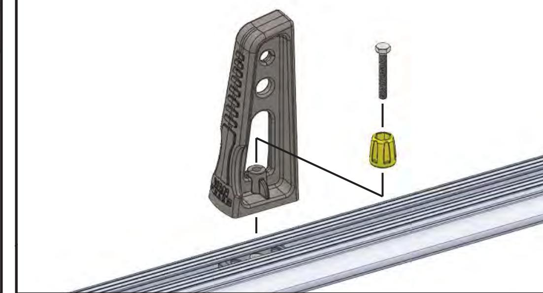
**3** Slide the load stops to the required position on the roof bar and tighten by hand. Once the load stops have been tightened by hand the supplied tool (MA6068) can be used to tighten further.
