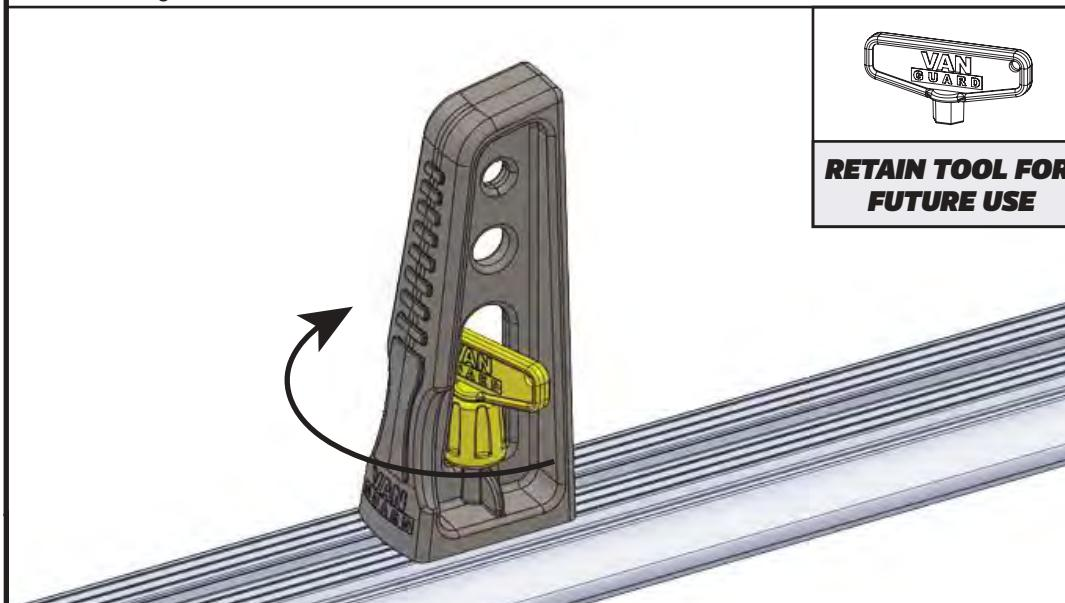
**4** If the load stop is removed from the roof bar remember to also remove the rail plate. The rail plate must not be left inside the roof bar when it's not in use.
