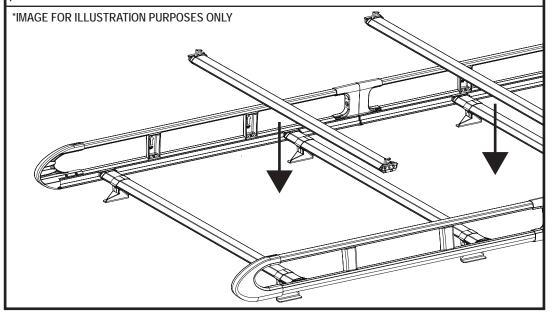
Assemble the roller spigot, M8 t bolt (FX4139) and M8 shakeproof washer together. Place the assembly into the roller. Slide the roller onto the spigot fitted in step 15, drop the other end into position and then tighten using the supplied tool (ME0182).
