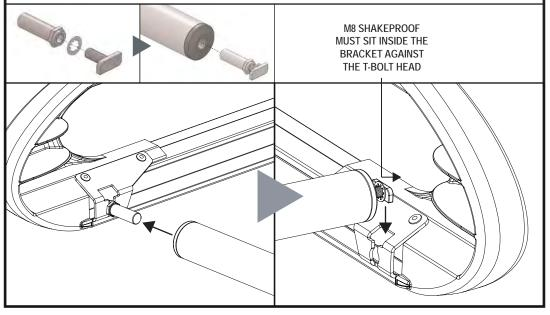
**15** Secure the roller spigot to the left hand roller bracket only using a M8 t bolt (FX4139) and a M8 shakeproof washer. Ensure that the shakeproof is on the inside of the roller bracket and that the spigot sits flush / straight. Tighten using the supplied tool.
