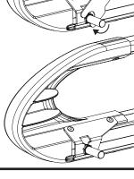
Assemble the roller spigot, M8 t bolt (FX4139) and M8 shakeproof washer together. Place the assembly into the roller. Slide the roller onto the spigot fitted in step 14, drop the other end into position and then tighten using the supplied tool (ME0182).
