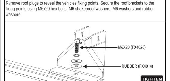
The following step is for vehicles with threaded insert fixing points. If fitting
