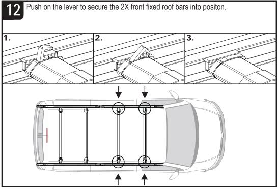
Place the remaining roof bars into position. See page 2 for the recommended distances between the roof bars. Once in position push on the lever to secure in place.
