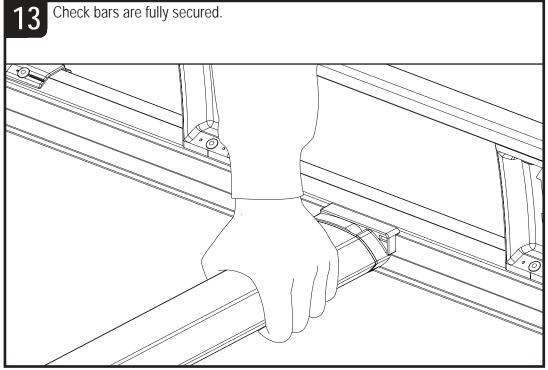
Once the product has been fitted check fixings and parts to ensure they have been fully secured and tightened. Check fixings and parts at regular intervals. Any damaged or worn parts must be immediately removed from the vehicle and replaced.
