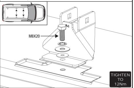
Secure the rear roof brackets by bolting down through the drilled fixing points using M8x30 hex bolts, M8 shakeproof washers, M8x25 washers and rubber washers. Secure under the roof using large rubber washers, M8x38 washers and M8 flange nuts.
