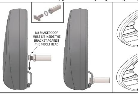
Assemble the roller spigot, M8 t bolt (FX4139) and M8 shakeproof washer together. Place the assembly into the roller. Slide the roller onto the spigot fitted in step 15, drop the other end into position and then tighten using the supplied tool (ME0182).
