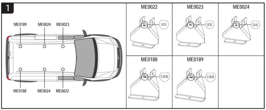
As there are no fixing points at the rear of the vehicle it's necessary to drill the roof to create 2X rear fixing points. Measure 155mm from the edge of the rear door opening and drill 2X fixing points (one either side) Ø8.2mm. It is recommended to drill a Ø4mm pilot hole first.
