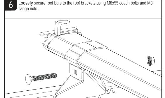
Place a flat object across the roof bars to ensure that they're level. If the roof bars sit level please skip to step 8. Due to the variance in some vehicles a spacer is supplied for the middle roof brackets. If the middle brackets are sitting too low please remove the middle brackets and re-secure using M8x30 hex bolts, spacer pads, M8 shakeproof washers, M8x25 washers and rubber washers.
