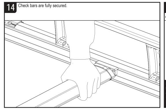
15 Once the product has been fitted check fixings and parts to ensure they have been fully secured and tightened. Check fixings and parts at regular intervals. Any damaged or worn parts must be immediatey removed from the vehicle and replaced.
