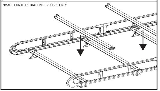
12 Assemble the roller spigot, M8 t bolt (FX4139) and M8 shakeproof washer together. Place the assembly into the roller. Slide the roller onto the spigot fitted in step 11, drop the other end into position and then tighten using the supplied tool (ME0182).
