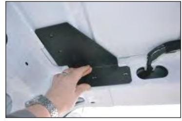
Loosely secure the front inner fixing brackets to the inside of the vehicle. Where a sliding door is present remove the 2X star drive screws, place front inner bracket in position and refit star drive screws as shown in fig.1. (Do not remove door rail bracket)
