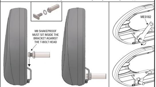
Assemble the roller spigot, M8 t bolt (FX4139) and M8 shakeproof washer together. Place the assembly into the roller. Slide the roller onto the spigot fitted in step 12, drop the other end into position and then tighten using the supplied tool (ME0182).
