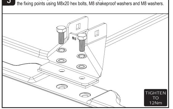
Remove roof plugs to reveal the vehicles fixing points. Secure the roof brackets to
