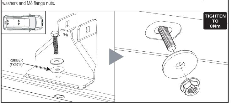
Remove roof plugs to reveal the vehicles fixing points. Secure the rear and middle roof brackets by bolting through
