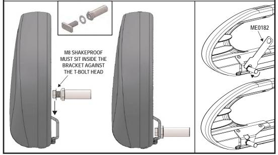
Assemble the roller spigot, M8 t bolt (FX4139) and M8 shakeproof washer together. Place the assembly into the roller. Slide the roller onto the spigot fitted in step 13, drop the other end into position and then tighten using the supplied tool (ME0182).
