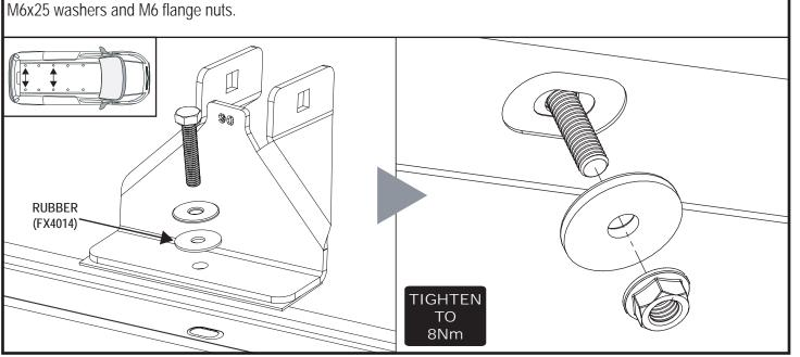
Remove roof plugs to reveal the vehicles fixing points. Secure the rear and middle roof brackets by bolting through the vehicles fixing points using M6x30 hex bolts, M6x20 washers & rubber washers. Secure under the roof using
