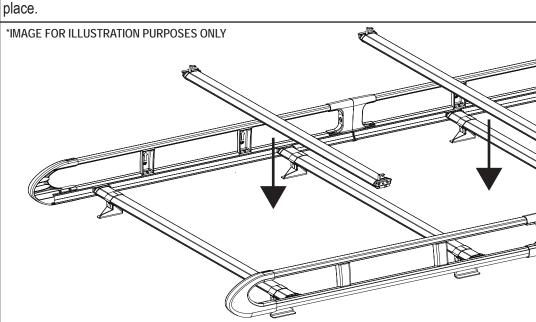
Place the remaining roof bars into position. See page 2 for the recommended distances between the roof bars. Once in position push on the lever to secure in
