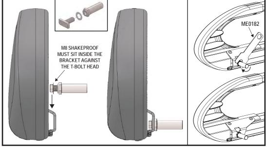
Assemble the roller spigot, M8 t bolt (FX4139) and M8 shakeproof washer together. Place the assembly into the roller. Slide the roller onto the spigot fitted in step 16, drop the other end into position and then tighten using the supplied tool (ME0182).
