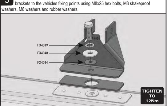
Stick the rubber pads to the underside of the roof brackets and secure the roof
