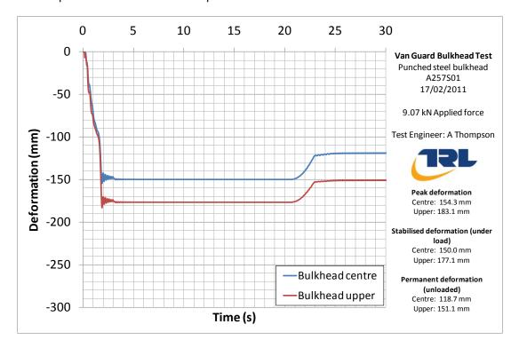
No sharp edges or other deformations were observed on the bulkhead during or after the test which may directly or indirectly result in injuries to the vehicle occupants.
